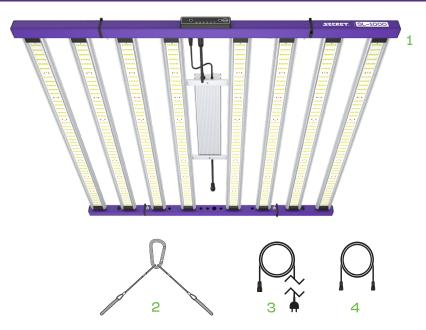
**SPECIFICATION SECRET SL-1000** Operating Voltage 100-277 VAC 50/60 Hz Operating Freq Input Current 8.33A @ 120V, 4.17A @ 240V, 3.16A @ 277V PPF (umol/s) 2900 **Energy Use** 1000 Watts (±5%) PPF/Watt (umol/J) 2.9 Operating Temp -4°F to 95°F (-20°C to 35°C) **BTU Output** 3412 43.31 x 43.31 x 3.54 Dimensions (in) Dimensions (mm) 1100 x 1100 x 90 Net Weight 20.42 lbs (13.8 kg) 5 Year Limited Warranty Q90 > 50,000 Hours Life Rating Certifications ETL, CE, DLC Hort Environment IP65, Wet Rated
